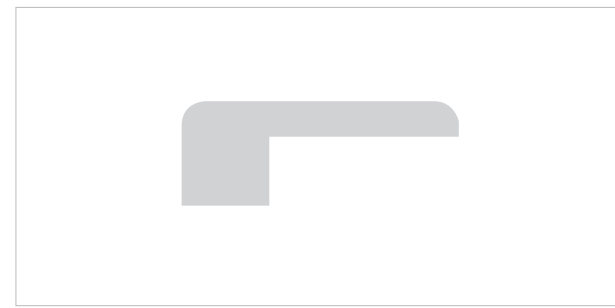
Mit Overlay Profile Section Produced from 12 mm MDF Panel.
