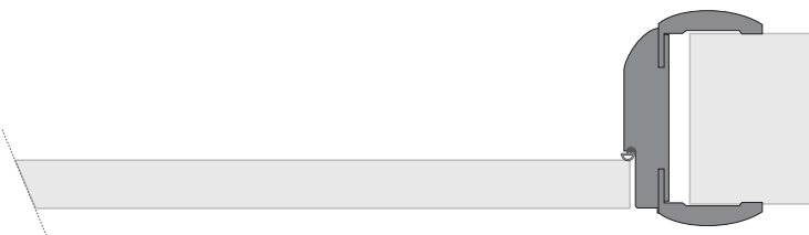
Rounded Frame - Rounded Architrave Combination
